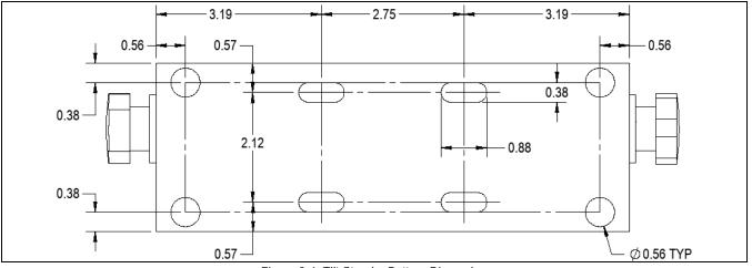
Figure 3-4. Tilt Stand – Bottom Dimensions
