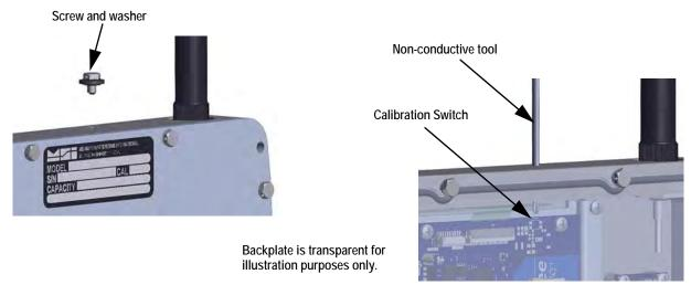
Figure 5-1. Press Configuration Switch
