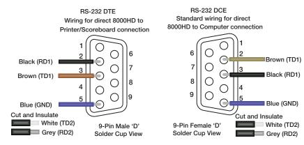
Figure 6-4. Communications Port 2 Wiring
