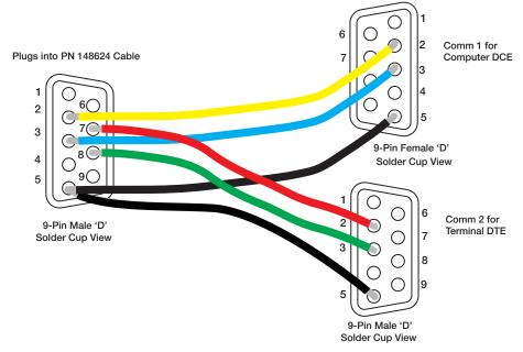
Figure 6-5. Connection with Y Adapter
