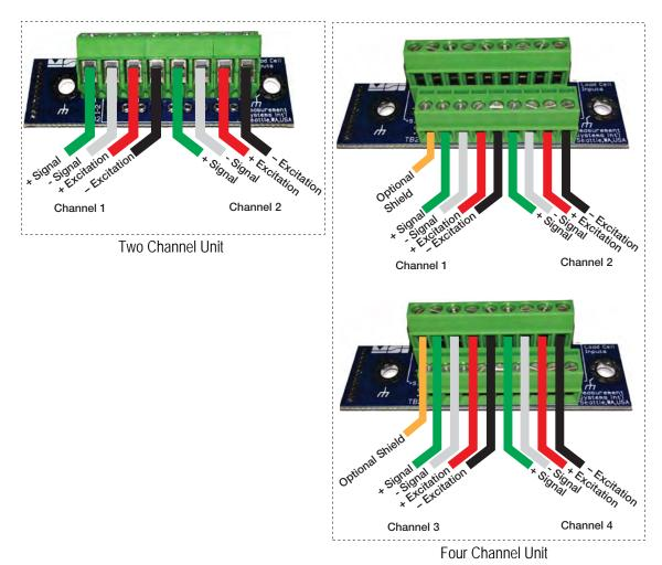
Figure 3-3. Wiring Diagram
