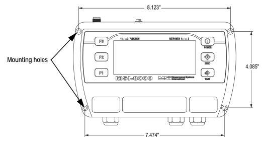
Figure 3-5. Mounting Hole Dimensions
