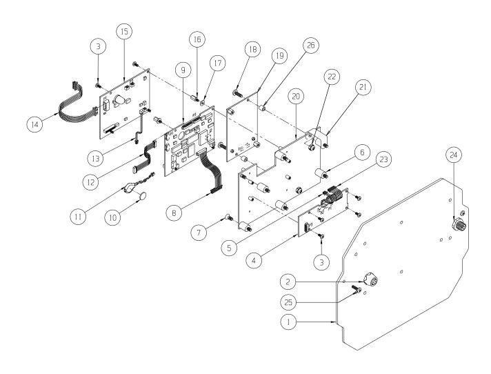
MSI-9300 Mid-section Assembly 500 - 10,000 lb (S-beam Load Cell)
