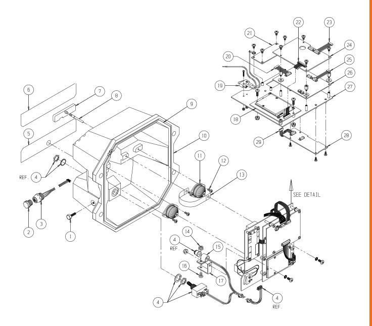
MSI-6260CS Mid-Section Assembly (500 - 10,000 lb) (S-Beam Load Cells)
